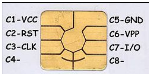
Gambar 5 Smart Card's pin contact
